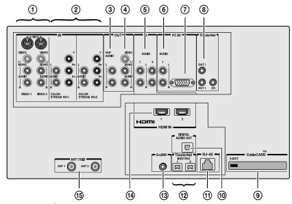
(1) VIDEO 1 IN and VIDEO 2 IN — Two sets of standard (composite) video and standard audio inputs plus optional S-video inputs for connecting devices with composite video or S-video output.
